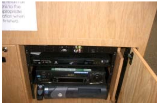
Figure 4 –Instructor station DVD and VHS source equipment. Source images are displayed via ceiling mounted
