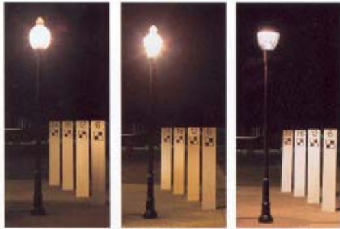
Figure 1.1 – Fixtures with cut-off optics not only reduce light pollution but can achieve greater illumination levels.
