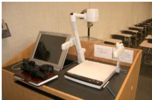
Figure 1 – Example of newer instructor media station with dedicated computer and document camera.
