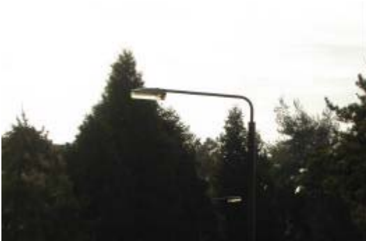
Figure 3.1 – Street lighting – low pressure sodium source emits light in only two wavelengths.
