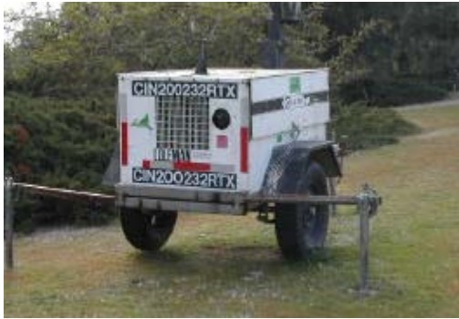
Figure 11.1 – Existing lighting consists of gas-powered construction floodlights.
