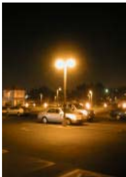
Figure 1.2 – Sodium light sources render all colors as gold, brown, or black, thus reducing visibility.
