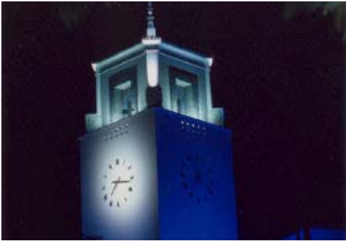
Figure 8.1 – Where beam distribution can be controlled so as to prevent directly illuminating sky, uplights are usable.
