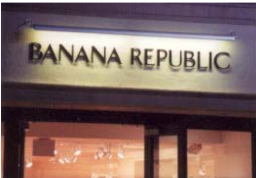
Figure 10.4 – Low profile fluorescent sign lighters can be used to downlight monument signage. (Cole SL)
