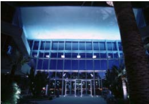
Figure 8.2 – Where uplights will not cause light pollution, they can be used to accent architecture.
